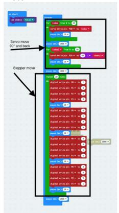
I downloaded the code onto the microbit. I tried it and nothing happened. I was using a 9V battery so I tested the voltage with my dad's multimeter. It was only 7.3V so I got a new battery. I tried again with the new battery but I still couldn't see anything working.
